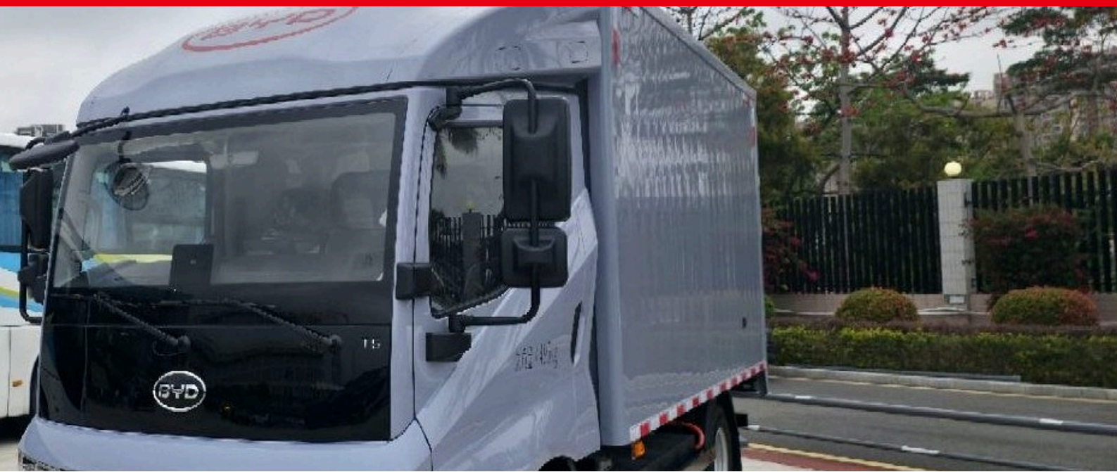
BYD T5 with box-van body — the 5-tonne hauler. Chassis-cab is the priced unit; box, refrigerated & drop-side bodies built to order.
